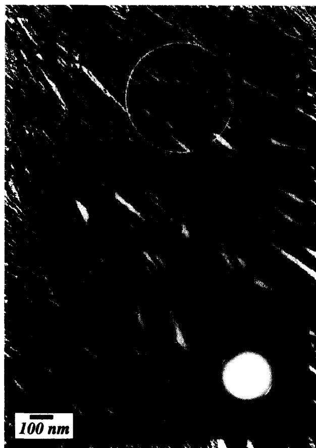
Figure 2 TEM observations of PEKK(I) edge-on lamellar morphology in spherulites grown from the melt at 230°C for 2 h. An ED pattern is also included
